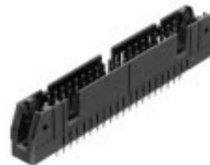
Pin Header without Latches Post Length .174 [4.42] for .093-.125 [2.36-3.18] Thick PC Board
