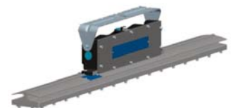
LSXW5 Mounting bracket Can be angled at 0°, 30°, 45°, 60° & 90°
