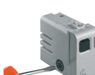
Fig. 3 3 rd phase: configuration RX receiver e.g. GW 14 821
