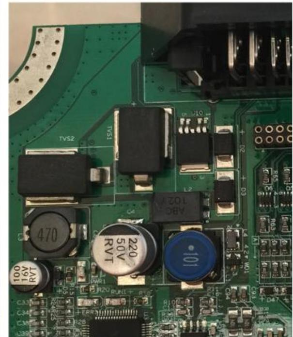
PANJIT uses automation vacuum soldering to assemble the DO-218AC package load dump TVS. Comparing with the traditional furnace soldering, automation vacuum soldering system helps reduce the soldering bias and void. The amount of the void effects the  $I_{pp}$  capability of the TVS, thus the lesser void on the die, the better IPP capability of the TVS; meanwhile the lower the thermal resistance is, the faster dissipation speed through thermal conduction.
