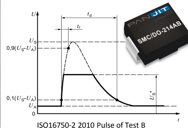
The testing voltage of ISO16750 Pulse B is 35% of the maximum polygonal voltage of Pulse A, thus the surge sustainability required for load Dump TVS is much lower. So for products that is tested based on ISO 16750 Pulse B, PANJIT recommends to use TVS assembled in SMC package (1.5KW/3.0KW/5KW).
