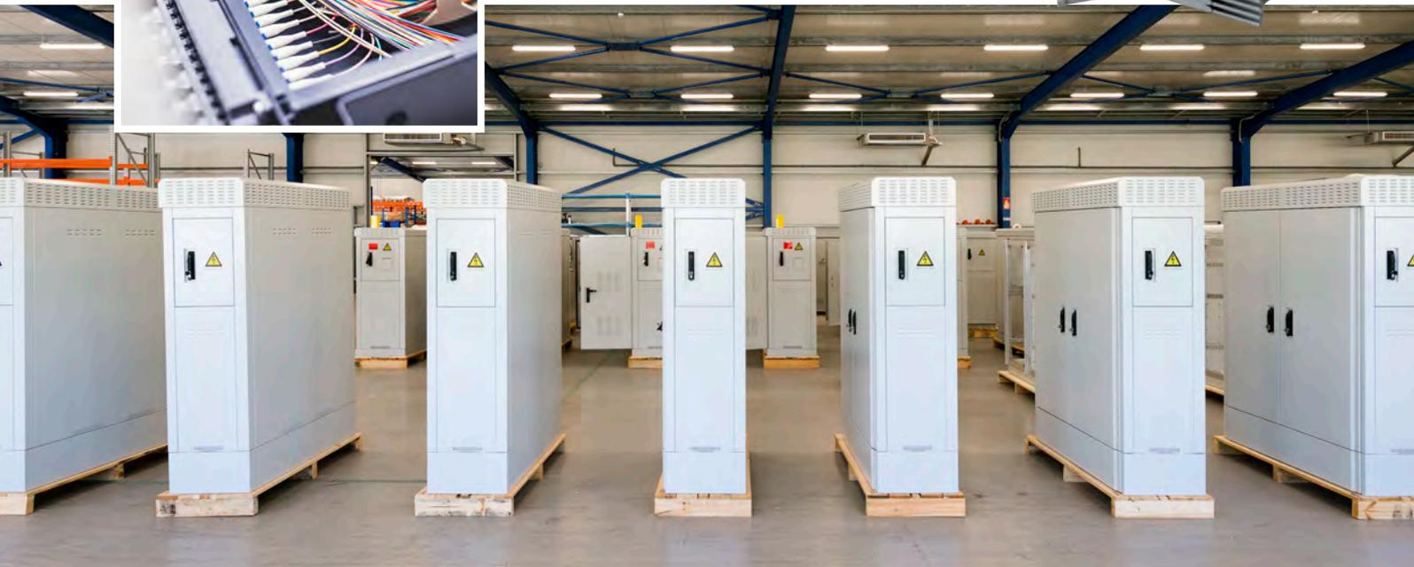
**Raycap telecommunication cabinets are designed for maximum flexibility and durability according to customer specifications and are manufactured in Europe.**
