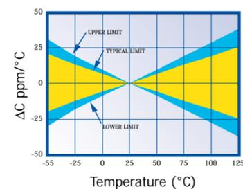
X7R capacitance vs temperature
