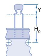
This style has been developed to provide a meniscus-free seating plane with a stress relieving form for auto-insertion.
