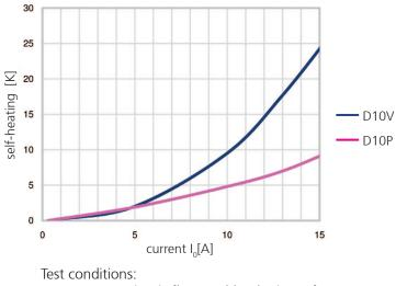
Measurement in air flow and lead wires of 1.5 mm<sup>2</sup>.
