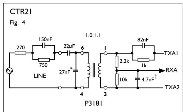
\* If components on line side to be unchanged for 600Ω/CTR21, compromise on 22nF.
