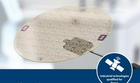
GH15 GaN process is optimized for applications up to 40GHz for high power, high PAE and high linearity.
