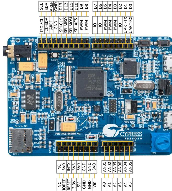
Table 3-2 shows full functions of the pins connected with the Arduino headers.
