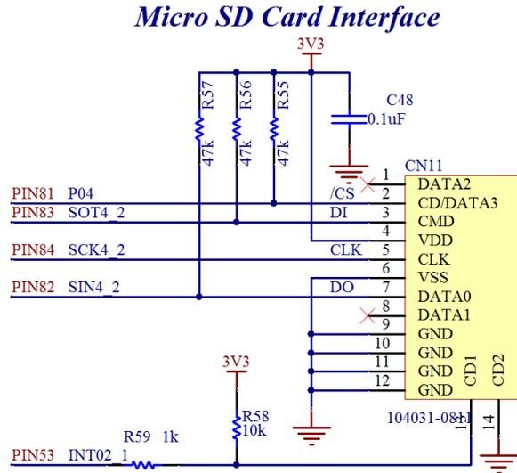
The pin arrangement of the Micro SD card is shown as below:
