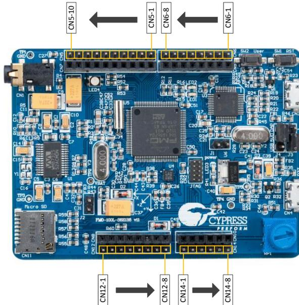
These additional GPIO interfaces make it easy for the user to access more GPIOs and peripherals, like the MFS (Multi-Function Serial), PWM and I2S. Table 3-3 shows details of the pins.
