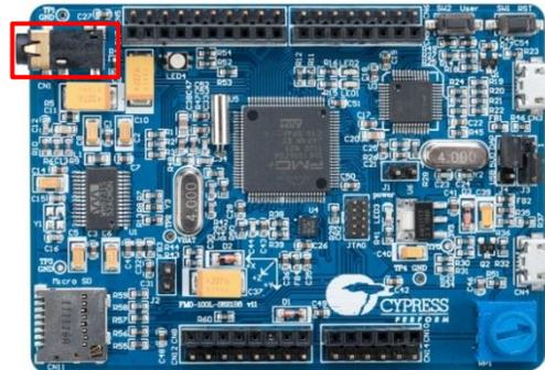
**Note:** Connect a headset with a 4-conductor phone plug (American Headset Jack) to CN1 for this test to function.
