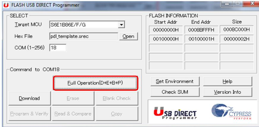
11. Reset the S6E1B8 by pressing the reset button (SW1) on the board, and click **OK**.
