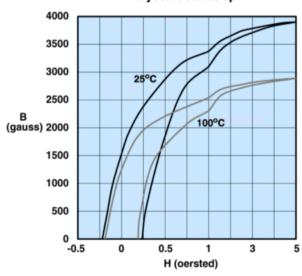
Measured on a 17/10/6mm toroid at 10kHz.
