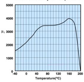
Measured on a 17/10/6mm toroid at 10kHz.
