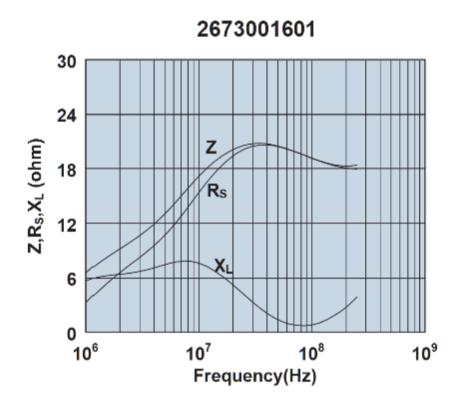
Impedance, reactance, and resistance vs. frequency.
