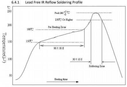
Remark: The peak temperature of soldering heat is  $260^{+5}_{-0}\ ^\circ\text{C}$
