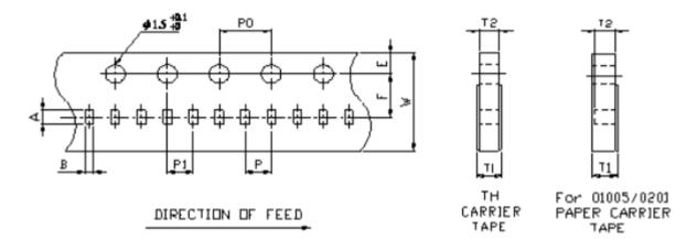
Remark: Pitch tolerance over any 10 pitches of Po is  $\pm$  0.2 mm
