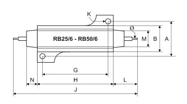
Fixed power wirewound resistors aluminium housed with faston leads
