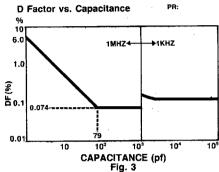
Dissipation Factor (Nominal capacitance greater than 330pF) **D** factor shall not exceed the values shown in Fig. 3.
