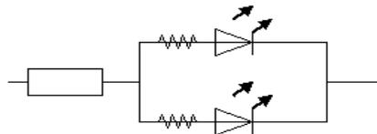
3. Sudden surge could damage the LED interior connections. Please design circuit with care so no sudden voltage surge or current surge will show when turning the circuit on or off.
