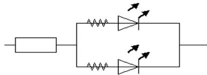
3. Sudden surge could damage the LED interior connections. Please design circuit with care so no sudden voltage surge or current surge will show when turning the circuit on or off.
