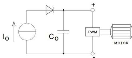
Conventional power supply: breaking power charges output capacitor C<sub>o</sub>
