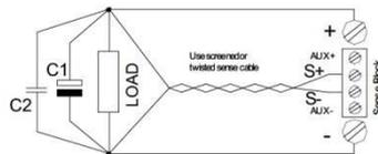
**Remote Sensing (2V per lead load, fig6)**
