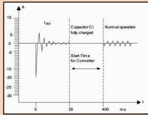
While connecting the HSD to the AC wire network its inrush current is limited to  $<5A_{peak}/3,5A_{effective}$ . The start capacitors are loaded after 20ms and the HSD actuates. After passing softstart the power supply is ready for operation after a total of  $\Delta t=400ms$ .
