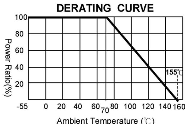
Power rating or current rating is in the case based on continuous full-load at ambient temperature of 70°C. For operation at ambient temperature in excess of 70°C, the load should be derated in accordance with figure of derating Curve.
