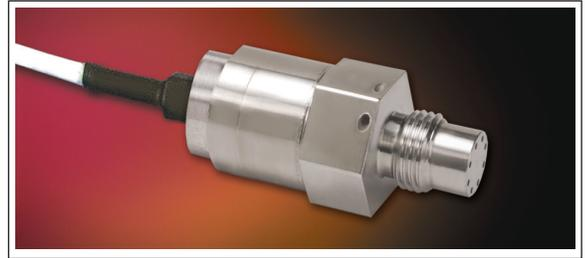
ETL-HT-375 Series transducers are miniature, threaded flush instruments. The sensing sub-assembly is protected from mechanical damage by a solid screen which has been shown to have minimal influence on the frequency response of the sensor. The ETL Series uses Kulite's Patented Leadless Technology. Incorporation
