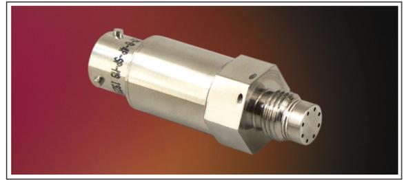
ETM-HT-375(M) CO Series transducers are miniature, threaded flush diaphragm instruments. They utilize a flush metal diaphragm as a force collector. Force is transferred to a solid state piezoresistive sensing element via a thin intervening film of non-compressible silicone oil. This sensing sub-assembly is protected from mechanical damage by a solid screen which has been
