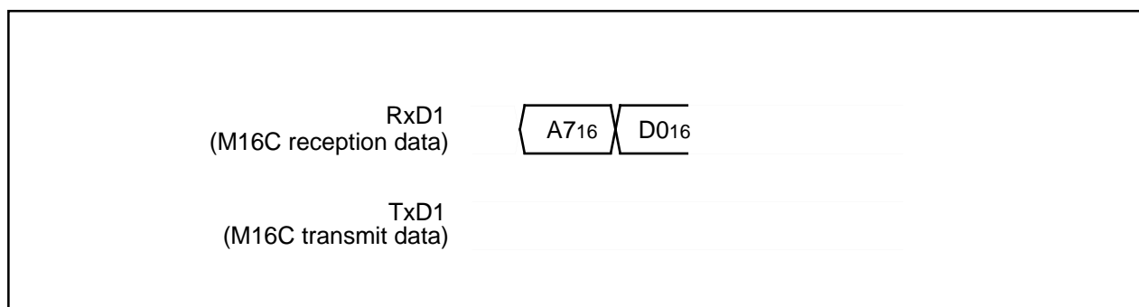
Figure 1.29.28. Timing for erasing all unlocked blocks
