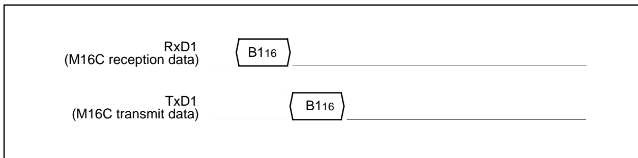
Figure 1.29.40. Timing of baud rate 19200
