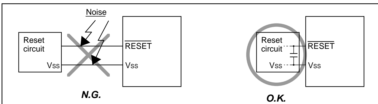
Figure 1.1.2. Wiring for RESET pin
