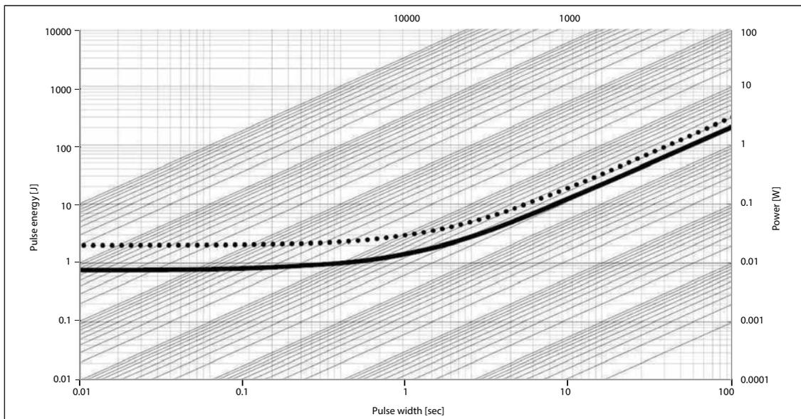
In this graph the max. & min. curve are shown as ••• and — for all resistance values, the area between the max. & min. curve is applicable. In case the Design Engineer requires a specific graph of a particular component it can be supplied on request.
