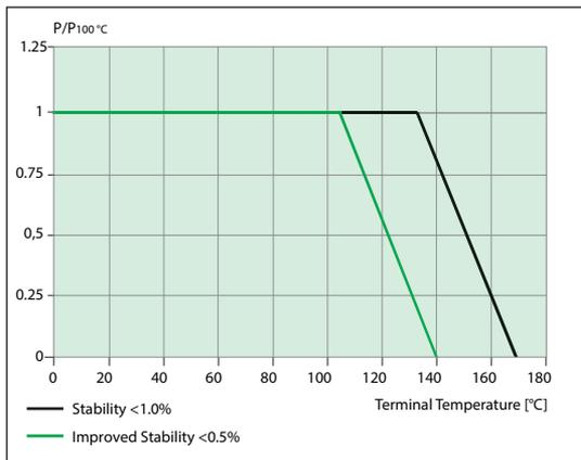
**TYPICAL POWER DERATING CURVE FOR RESISTOR WHEN FULL POWER IS AT 70°C**
