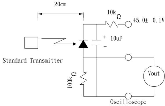
Fig.-3 Measuring System
