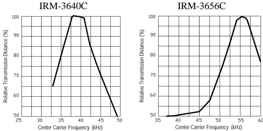
Fig.-9 Relative Transmission Distance vs. Center Carrier Frequency
