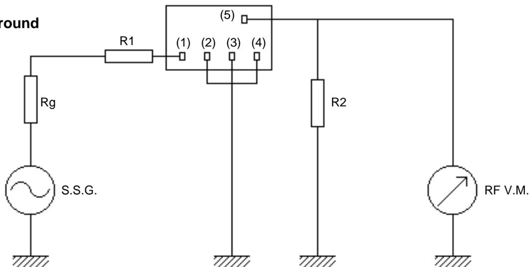
$$R_g + R_1 = R_2 = \text{Input / output impedance}$$
