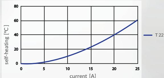
The characteristic curve in the diagram is measured with a thermal switch without any insulation in an oil bath.
