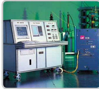
Characteristics Test / VCB Characteristics Test
