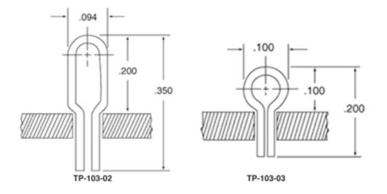
\*Note: Leads flared to provide retention in the printed circuit board.
