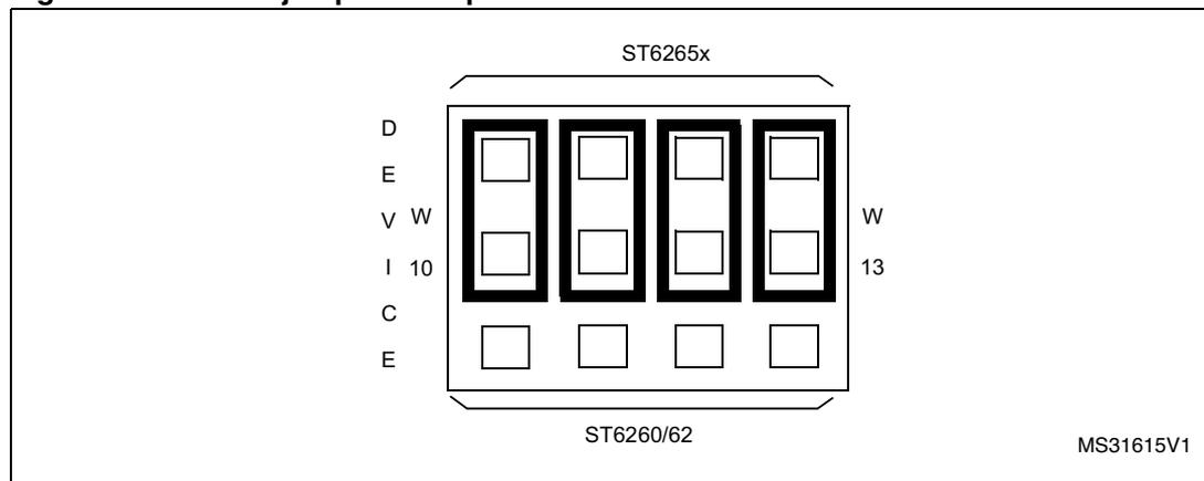
3. Select the USER mode using the jumpers marked W1 and W2 (marked 18 on the [Starter kit board diagram on page 13](#)), as shown in the diagram below:
