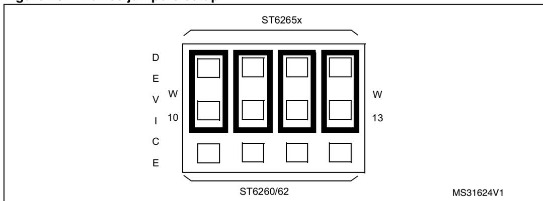
3. Select the PROG mode using the jumpers marked W1 and W2 (marked 18 on the [Starter kit board diagram on page 13](#)), as shown in the diagram below:
