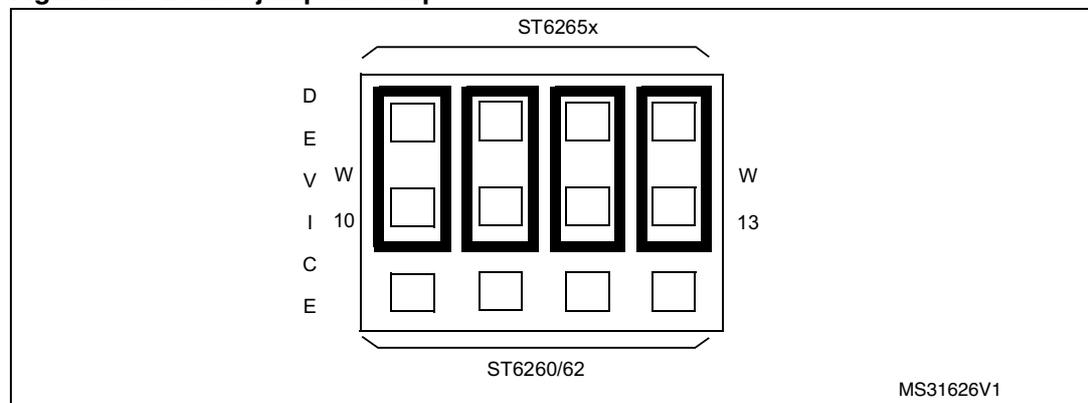
4. Select USER mode using the jumpers marked W1 and W2 (marked 19 on the [Starter kit board diagram on page 13](#)), as shown in the diagram below:
