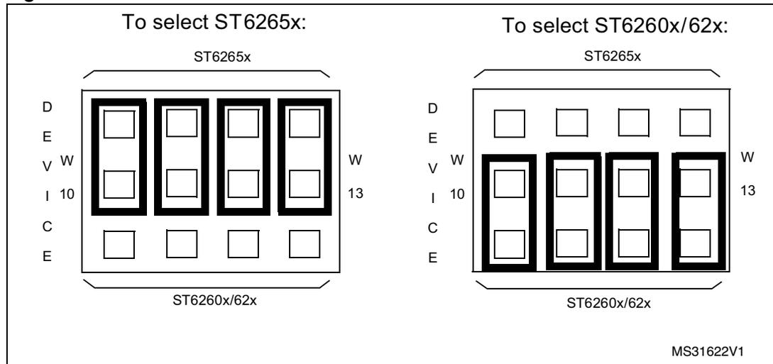
5. Select the PROG mode using the jumpers marked W1 and W2 (marked 18 on the [Starter kit board diagram on page 13](#)), as shown in the diagram below:
