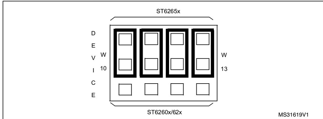
3. Select the USER mode using the jumpers marked W1 and W2 (marked 18 on the [Starter kit board diagram on page 13](#)), as shown in the diagram below:
