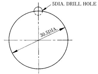
Note: The 5mm hole is used to stop whirl. If nameplates are not used or nameplate does not have any whirl-stop, the hole is not required.
