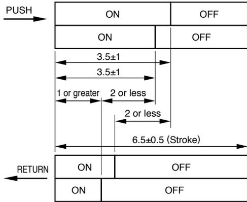
Note: Operate the plunger within the speed that the plunger can follow.
