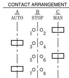
Note: when the switch is used in a DC circuit, connect odd number to ⊕, and even number to ⊖.
