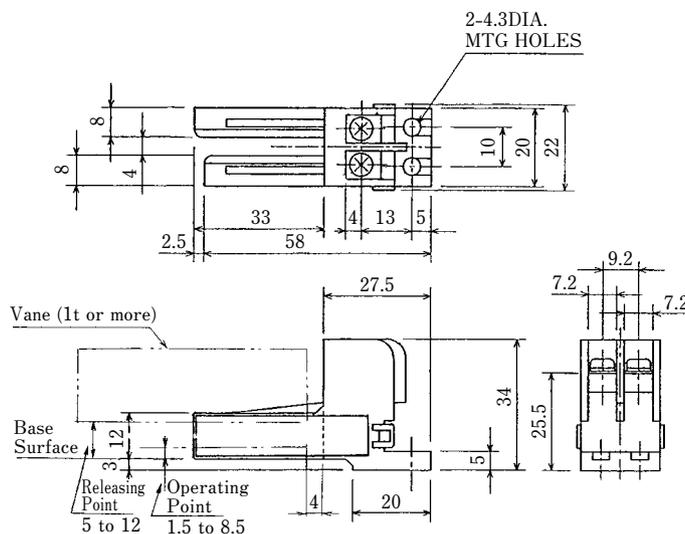
Note: When switch is used in a DC circuit, connect terminal 1 to ⊕ and number 2 to ⊖.
