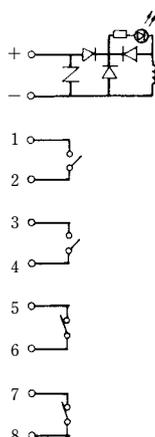
Note: When used in a DC circuit, connect the odd number terminals to ⊕ and even number terminals to ⊖.
