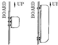
(a) Where placing board vertically (Standard)
