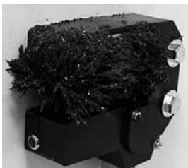
Adhesion of iron particles (60g)
