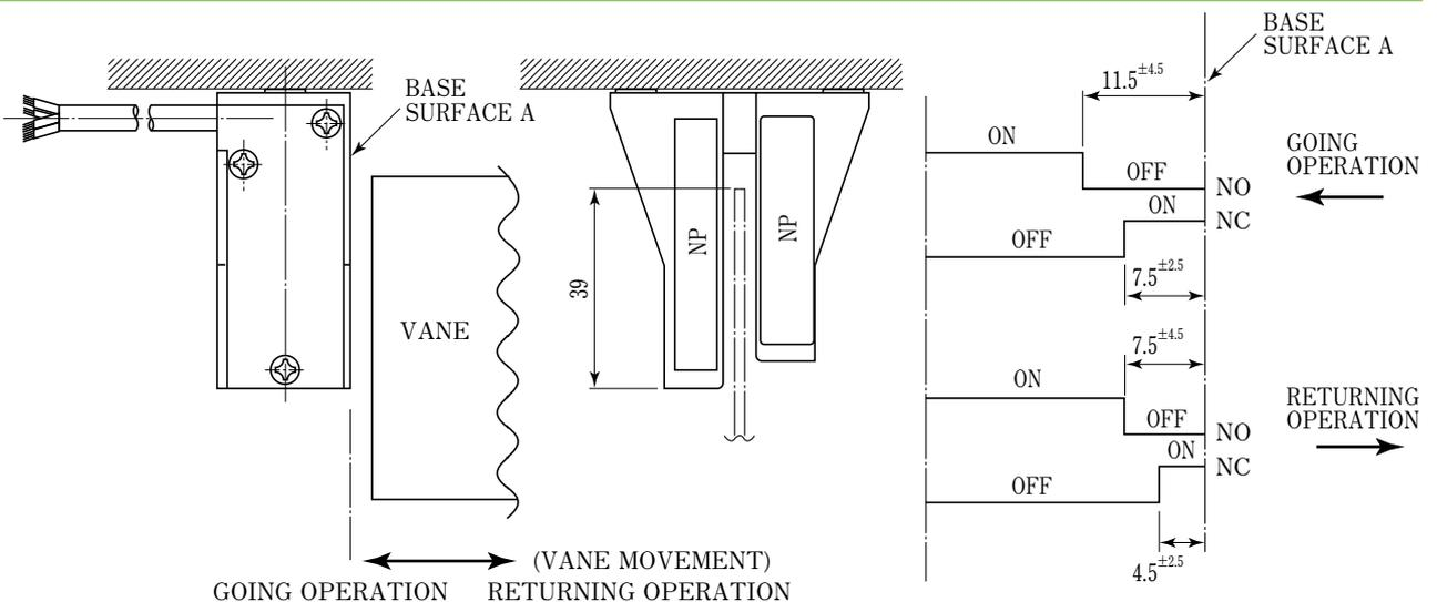
**Recommended vane material: SPCC&SPHC (Magnetic material), Thickness: 1.2mm, width 50mm or greater
