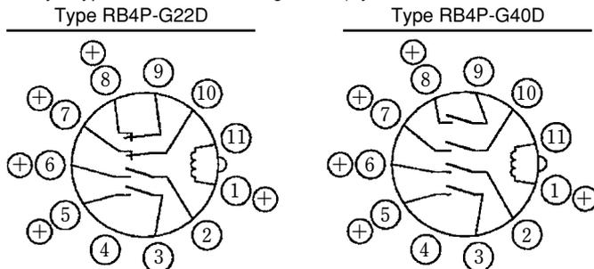
· Use coils and contacts according to the above polarity.
