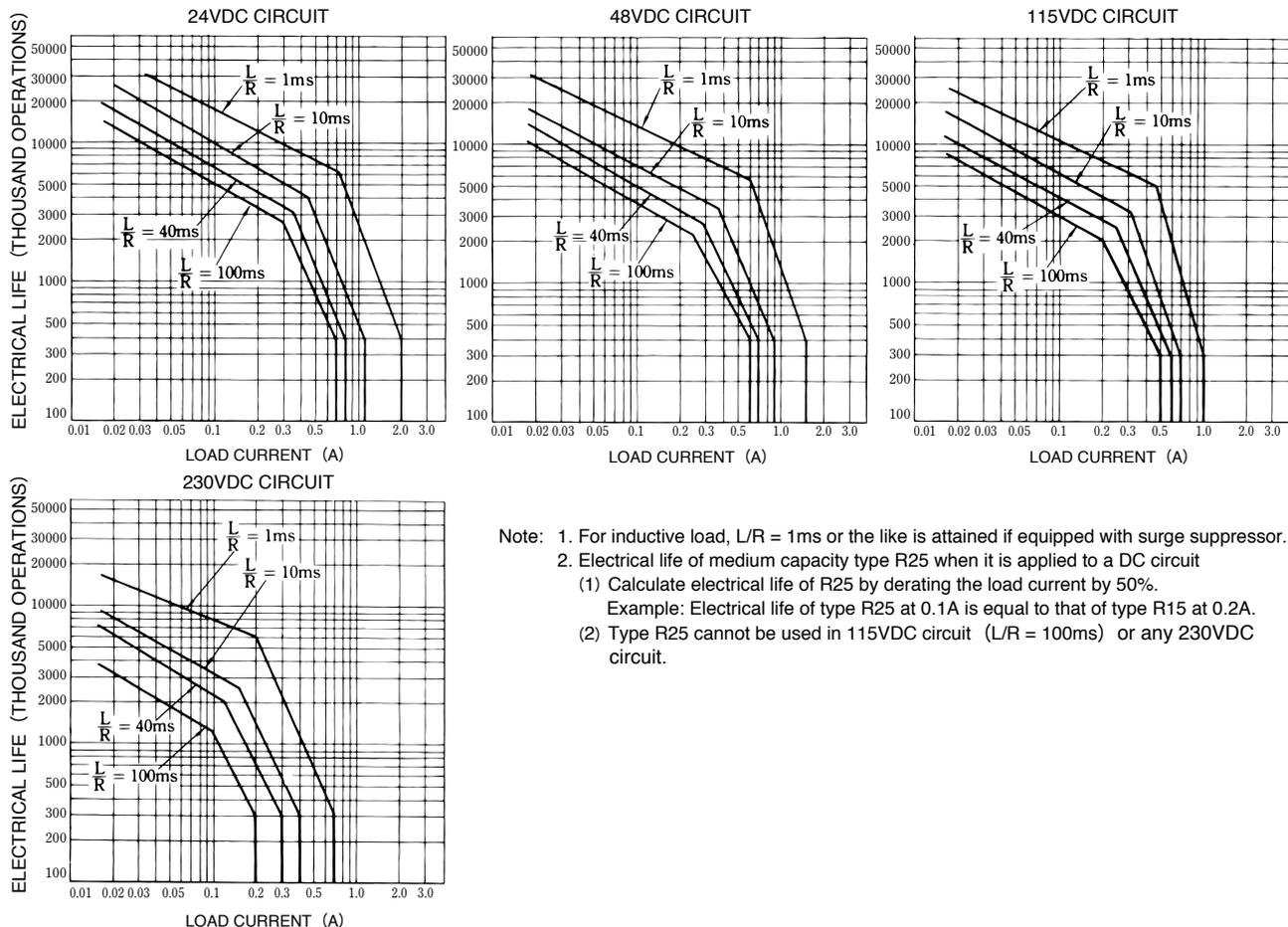
Note: 1. For inductive load, L/R = 1ms or the like is attained if equipped with surge suppressor.
