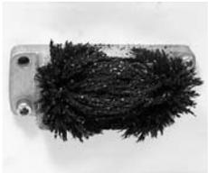
Adhesion of iron particles (30g)
