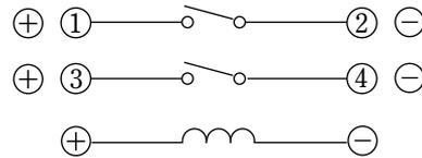
Terminal Markings and Contact Arrangement (Top View)
