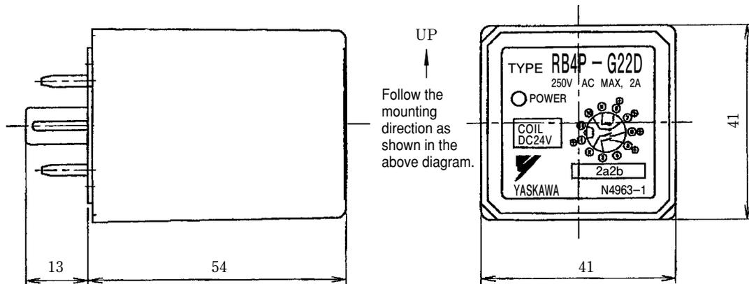
Relays Type and Contact Arrangement (Symbols and Terminal Markings: BOTTOM VIEW)
