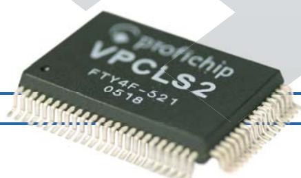
The VPCLS2 ASIC is a complete single chip solution for PROFIBUS DP. It provides 32 I/O points, which can be set to input, output or diagnostics (in groups of 8 bits). No additional microcontroller or software is needed. Therefore this ASIC is the ideal solution for simple digital field devices. The VPCLS2 is pin-compatible to the LSPM2 ASIC from Siemens.
