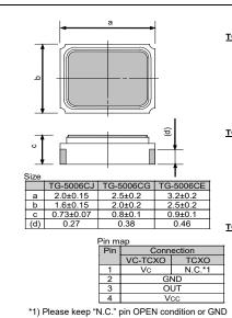
connection. "N.C." pin doesn't work as a ground pin
