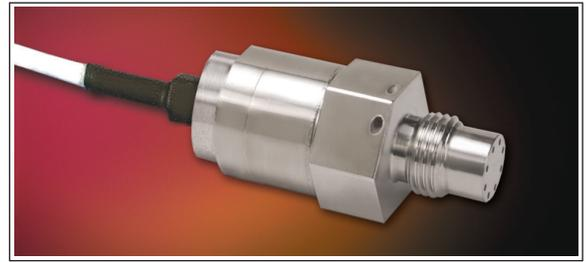
ETM-HT-400-375 Series transducers are miniature, threaded flush diaphragm instruments. They utilize a flush metal diaphragm as a force collector. Force is transferred to a solid state piezoresistive sensing element via a thin intervening film of non-compressible silicone oil. This sensing sub-assembly is protected from mechanical damage by a solid screen which has been
