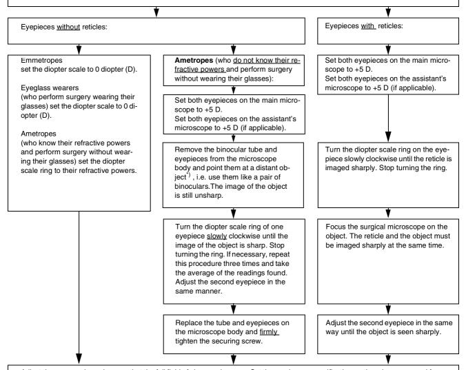
Adjust the eyecups in such a way that the full field of view can be seen. Set the maximum magnification on the microscope and focus on the object. Set the working magnification required. When the magnification is changed, the focal plane is retained, but the depth of field changes.
