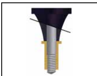
STEP 1 The fastener is threaded onto the pull-up stud of an installation tool.
