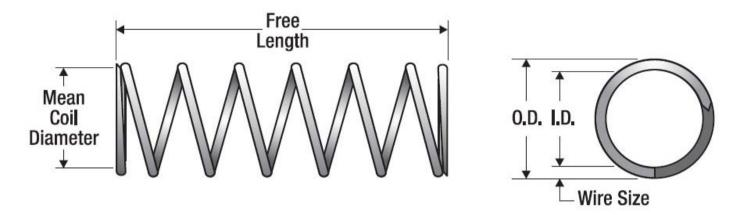
Regular compression spring in music wire with 8.50 total coils and closed/ground ends. This spring features an O.D. of 0.375in, an I.D. of .323in, a spring rate of 2.4. This spring is unfinished and gold irridite or zinc are available for an additional charge. Adding a finish will extend the lead time by 4 days.
