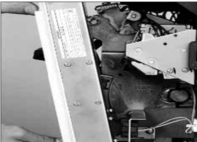
6. Mate pin connectors.
