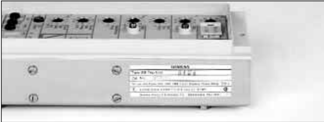
4. Check label on side of trip unit.
